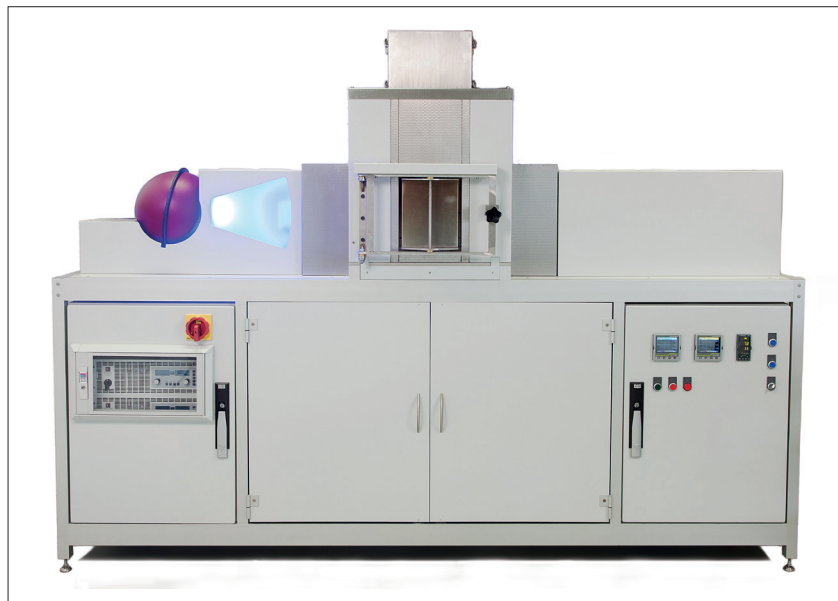
Fig. 3 Thermo-optical measuring (TOM) device TOM air used for measuring the uniaxial viscosity of the materials
