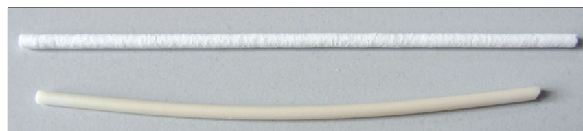
Fig. 6 Solid rods (diameter 3,3 mm) made out of RAMUL-HT (top) and a benchmark material (bottom) after five kiln cycles at a dwell temperature of 1600 °C
