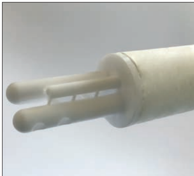
Fig. 13 Measuring tips for temperatures and gases made of alumina by 3D printing joined to the head of O-CMC lances
