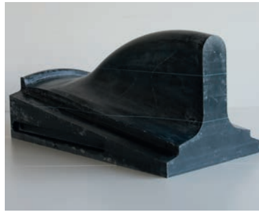
Fig. 3 b Plastic positive mould for laminating with pre-cut prepregs
