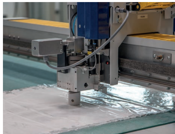
Fig. 5 Automatic cutting table for pre-cutting of individual coupons from the prepreg roll
