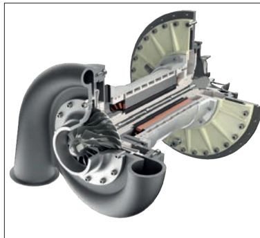
Fig. 14 Schematic drawing of a micro gas turbine including the demonstrator "stator" on the front side (Copyright Euro-K)
