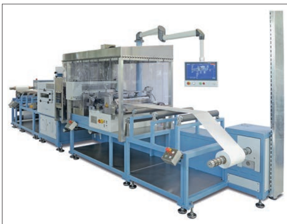
Fig. 4 Continuously operating roll-to-roll machine for production of prepregs by impregnation of oxide slurries (Copyright: Mathis AG)
