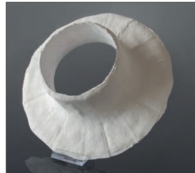
Fig. 15 Laminating study of a stator for micro gas turbines made of woven silica fabric and \text{Al}_2\text{O}_3\text{-SiO}_2 matrix
