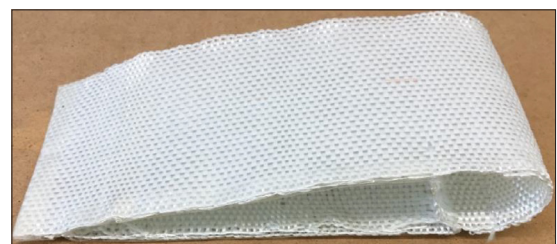
Fig. 8 First preform produced on a laboratory loom
